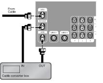
Note: When you use a converter box with your TV, there may be features that you can not program using the remote control, such as programming your favorite channels and blocking channels.
