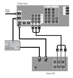
Caution: If you want to record one channel while watching another channel, a splitter (not included) must be added between the cable and ANT-A. One output of the splitter goes to ANT-A and the second output is connected to IN on the cable converter box.
